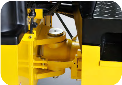
Articulated steering with a maintenance-free hitch and steering cylinder reduces maintenance
