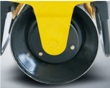
Thick drum shells for longer drum life.
